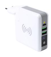
Multifunctional power bank / travel adapter with changeable wall plugs for USA, Europe, UK and Australia. With 6700 mAh battery, built-in wireless charger (5W), 2 USB and 1 USB-C (max. output 2400 mA) charger ports.
